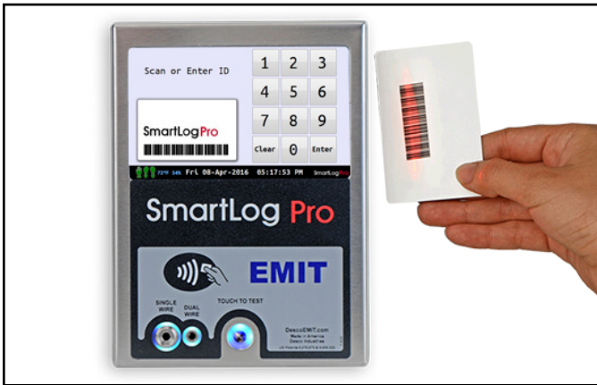
Figure 19. Using the barcode scanner
