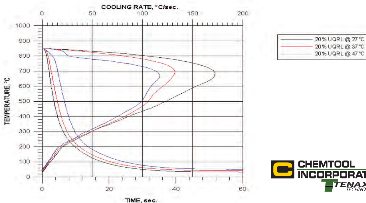
Figure 2 ● Temperature Effect on Cooling and Cooling Rate for UCON™ Quenchant RL Agitation Rate = 15 L/min.
