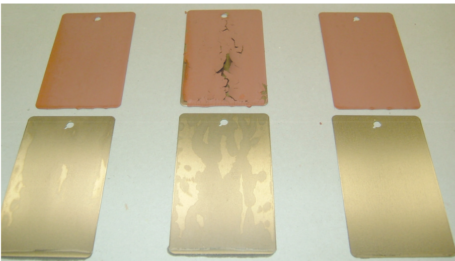
Paint Adhesion Test Method: R35 coupons dipped in respective rust preventatives, cured 24 hours. Top panels were sprayed with MIO shop primer and allowed to cure 24 hours. Bottom panels were not primed. Competitive Fluids on four right 4 panels. WeRP 6 on two left panels.
