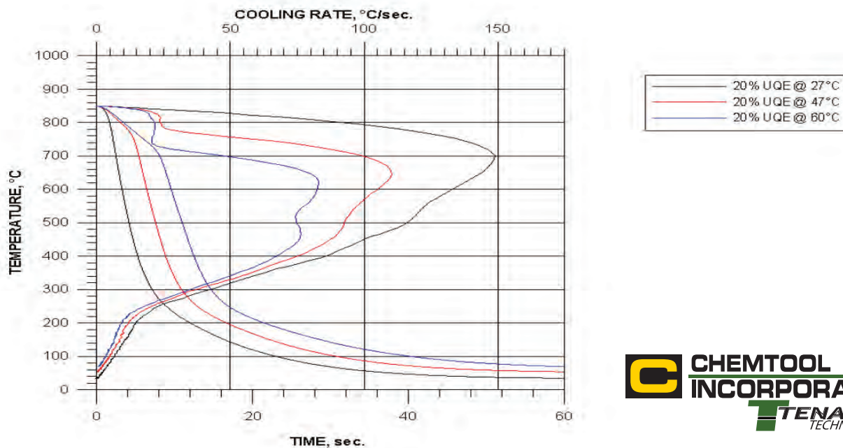
Figure 2 • Temperature Effect on Cooling and Cooling Rate for UCON™ Quenchant E Agitation Rate = 15 L/min.
