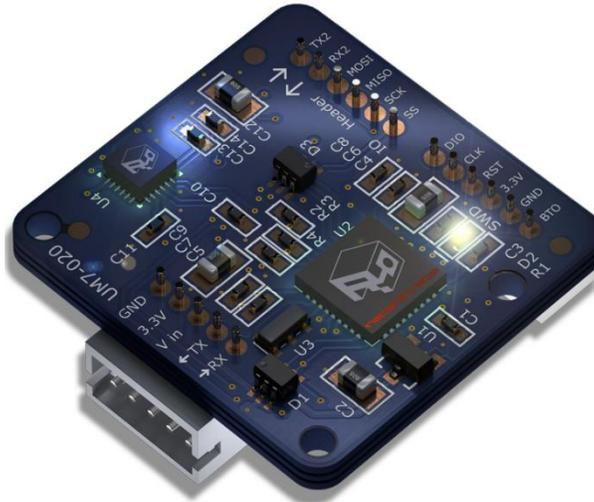
The UM7 is a 3rd-generation Attitude and Heading Reference System (AHRS) that takes advantage of state-of-the-art MEMS technology to improve performance and reduce costs. Like its predecessors, the UM7 combines triaxial accelerometer, rate gyro, and magnetometer data using a sophisticated Extended Kalman Filter to produce attitude and heading estimates.
