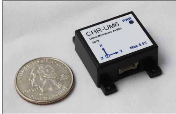
The UM6 simplifies integration by providing a number of automatic calibration routines, including rate gyro bias calibration, magnetometer hard and soft iron calibration, and accelerometer "zeroing" to compensate for sensor-platform misalignment. All calibration routines are triggered by sending simple commands over the serial interface.
