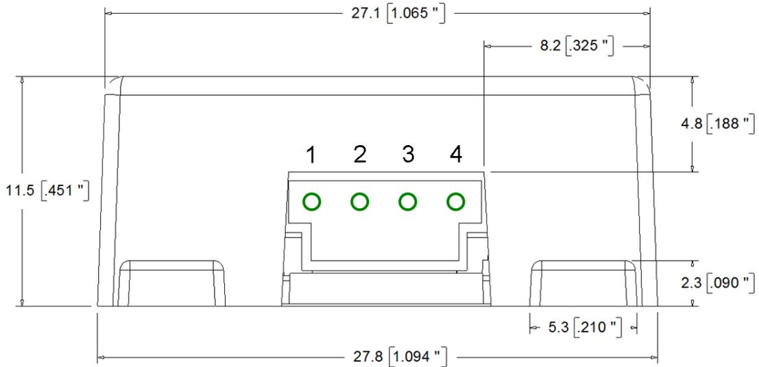
Part number A98655-ND from Digi-Key is a compatible connector for the 4-pin side output of the sensor (compatible connecting cables are also available from CH Robotics).
