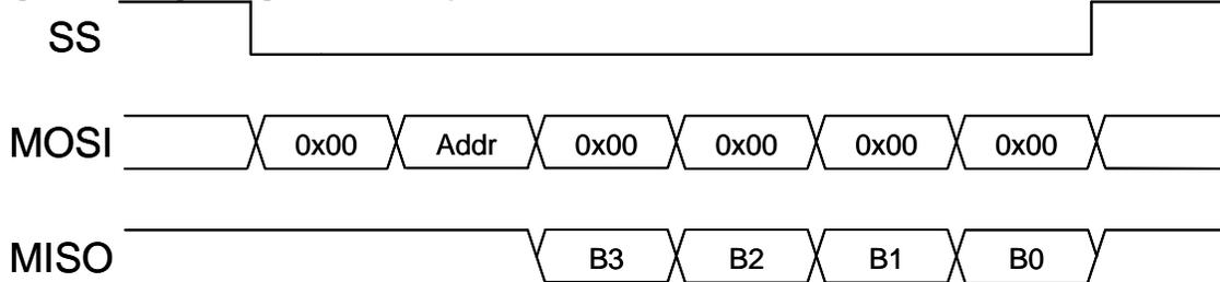
**Figure 3 - Multiple Register Read Operation**
