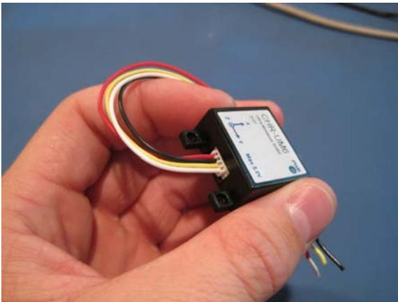
**Figure 7 - 4-Pin Side Connector**
