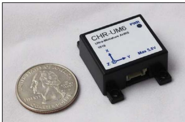
GPS modules to provide position, velocity, course, and speed information. Communication with the UM6 is performed over either a TTL (3.3V) UART or a SPI bus.
