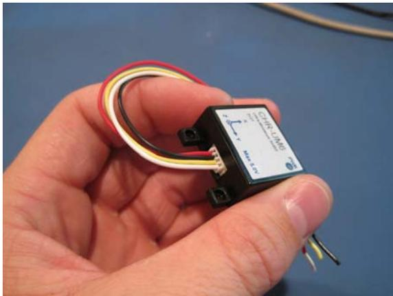
**Figure 7 - 4-Pin Side Connector**
