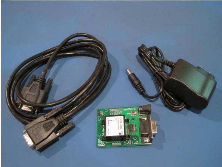
**Figure 1 - Serial Breakout Board Kit**
