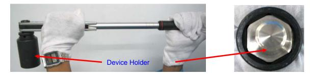
3. Move the device holder in direction of arrow until the cap is inserted and hex base is covered as shown in step 4.
