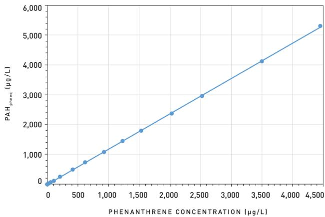
*UviLux PAH+ sensor dose-response curve to phenanthrene, demonstrating the excellent linearity ( $R^2 = 0.99998$ ) that can be achieved across the full range from 0 - 4500 µg/L, with integrated absorbance correction*
