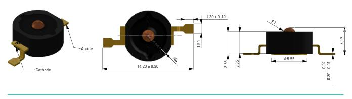
All dimensions are in millimeters. Unless noted otherwise, all dimensions have a tolerance of ± 0.05 mm.
