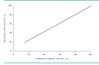
Test Conditions: Case Temperature (T<sub>c</sub>) = 25 °C
