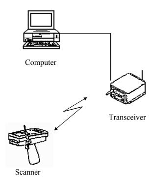
This entire system is configured to operate within warehouse buildings. Some internal antennae may be necessary to allow uninterrupted communication between the bar code scanners and the base station within the building. The base station transceiver will be networked to directly to the server. Data will be transferred via RF between bar code scanners and the base station. The server will also be networked to other Family Housing terminals.
