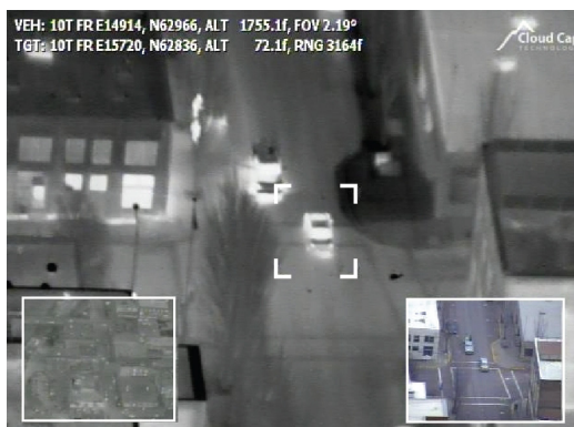
ViewPoint with video on map (left) and picture-in-picture display (right) simultaneously showing MWIR, LWIR and EO imaging and object tracking.
