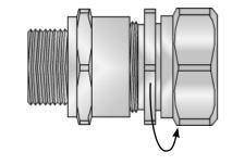
3. Fit the gland into the equipment and fully tighten the Entry Item (1).
