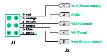
J1 and J2 connectors must not be used for frequency vibration measurements.
