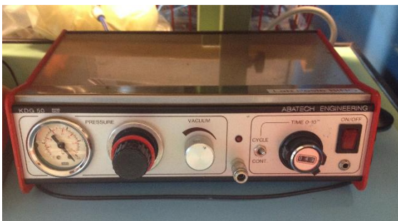
Figure 5: dispenser control panel
