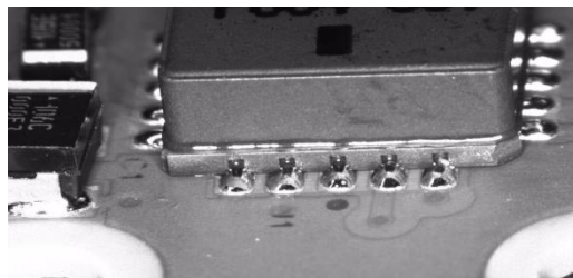
Figure 12: pads are well covered with melted solder
