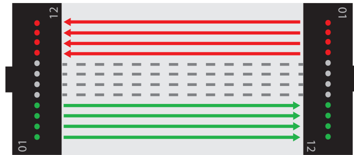
Figure 2: 40GBASE-SR4 (40GBE) and 100GBASE-SR4 (100GBE) full duplex operation on eight fibers
