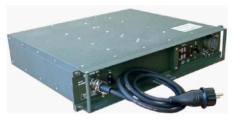
The BC 1500 RM 28V input current is power factor corrected and designed for optimum adaptation to weak power sources such as portable generators. The efficiency is very high due to the soft switching converter technology. The BC 1500 RM 28V is intended for mounting in 19" rack systems and occupies 2U (88mm) (3.5") height.
