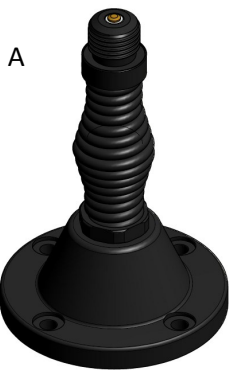
A NATO 4-hole Spring 4 x M10 or 3/8" Bolts on 114mm (4.5in) PCD Base diameter 140mm (5.5in) Base height 215mm (8.5in)
