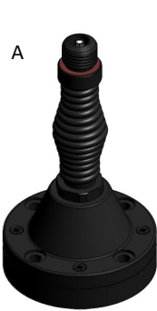
A NATO 4-hole Spring 4 x M10 or 3/8" Bolts on 114mm PCD Base diameter 140mm (5.5in) Base height 240mm (9.5in)
