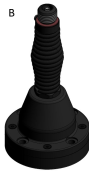
B NATO 4-hole Spring GPS 4 x M10 or 3/8" Bolts on 114mm PCD Base diameter 140mm (5.5in) Base height 280mm (11in)
