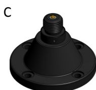
C NATO 4-hole Rigid 4 x M10 or 3/8" Bolts on 114mm PCD Base diameter 140mm (5.5in) Base height 100mm (4in)
