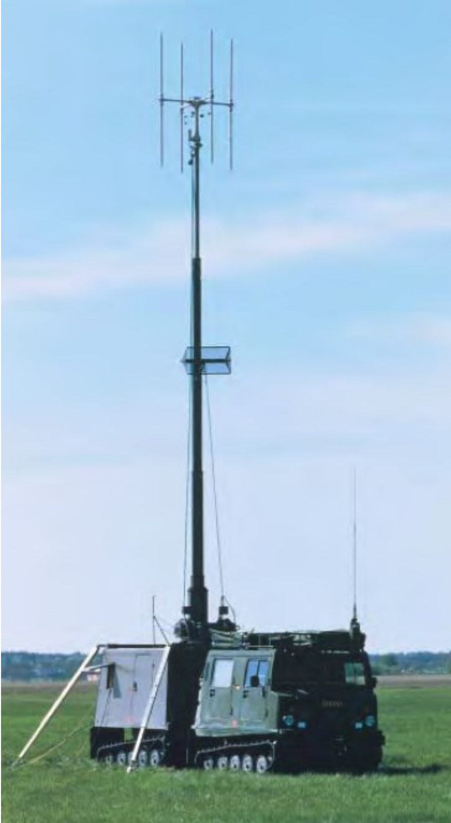
TM 300/18-2.8 mast integrated into Swedish Army Over-Snow Vehicle
