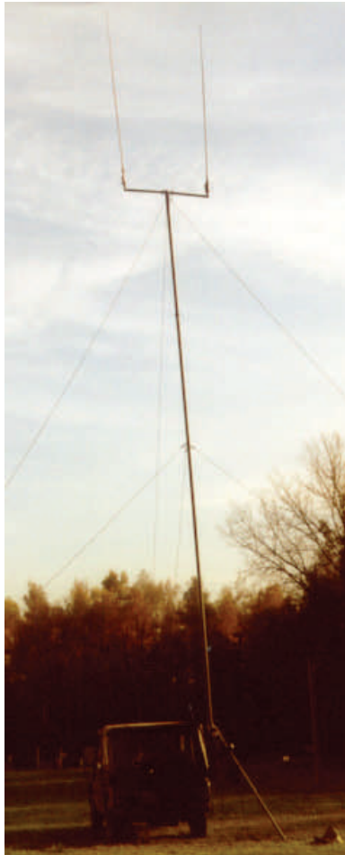
Sketch 2: 2 antennas on ULM-11/QESH mast
