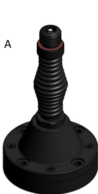
NATO 4-hole Spring 4 x M10 or 3/8" Bolts on 114mm PCD Base diameter 140mm (5.5in) Base height 240mm (9.5in)
