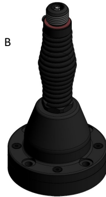
NATO 4-hole Spring GPS 4 x M10 or 3/8" Bolts on 114mm PCD Base diameter 140mm (5.5in) Base height 280mm (11in)
