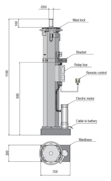
The hexagonal sections move inside each other on plastic guideways which provide the masts with excellent stability and torsional resistance.
