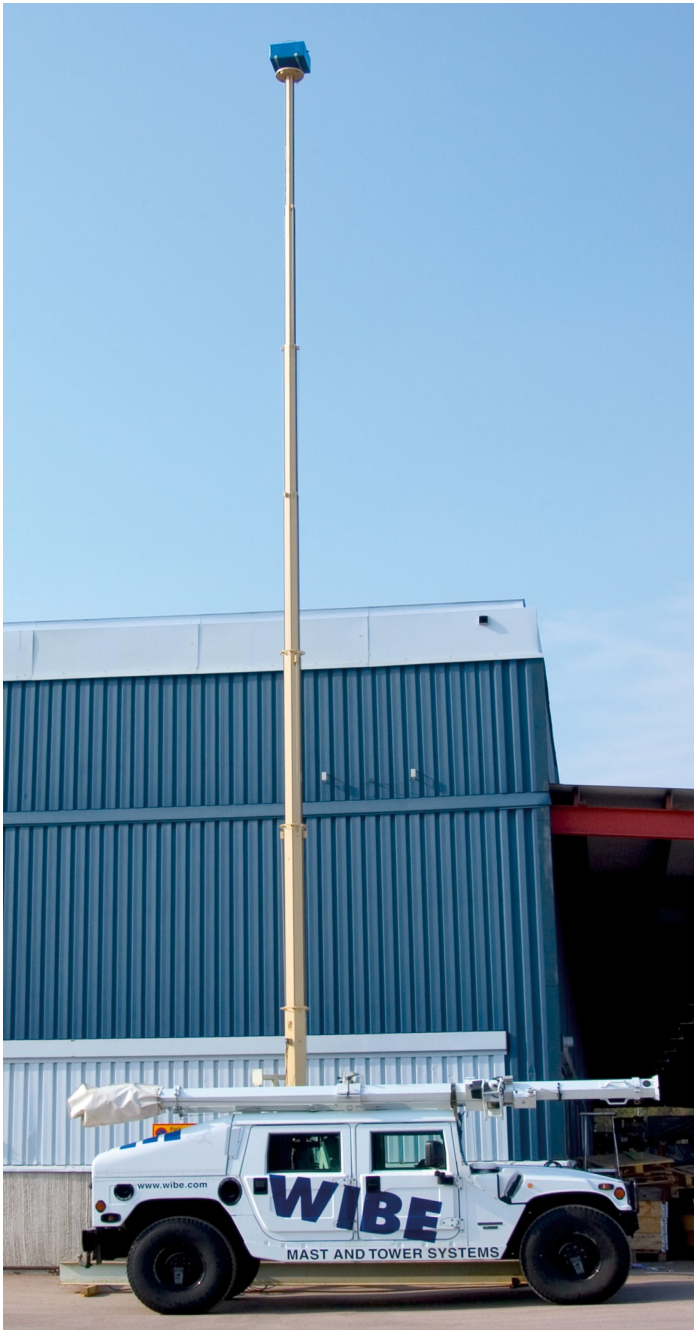
Fully deployed un-guyed mast
