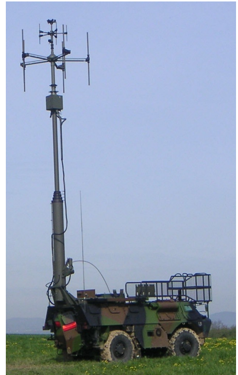
Mast elevated in the self-supporting (un-guyed) position
