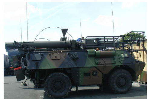
Mast in the horizontal (stowed) position during transportation
