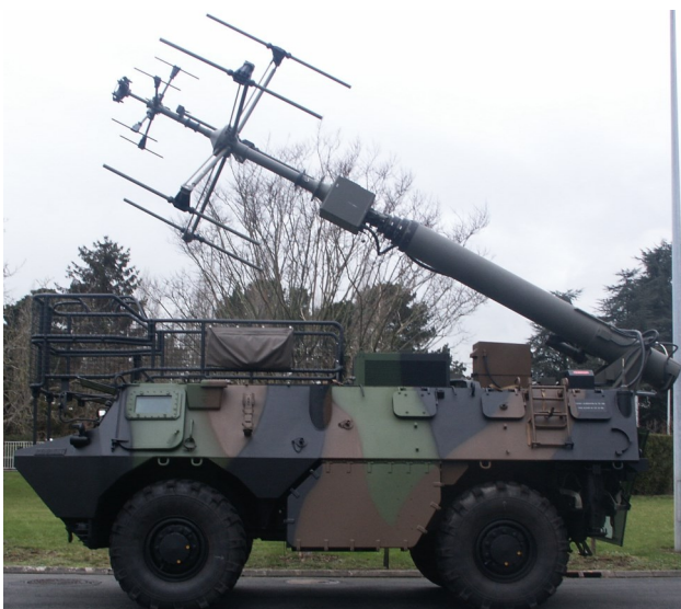
Automatic tilt from the horizontal storage position during mast deployment
