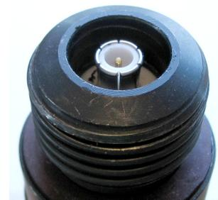
Picture of CEF connection on top of the base
