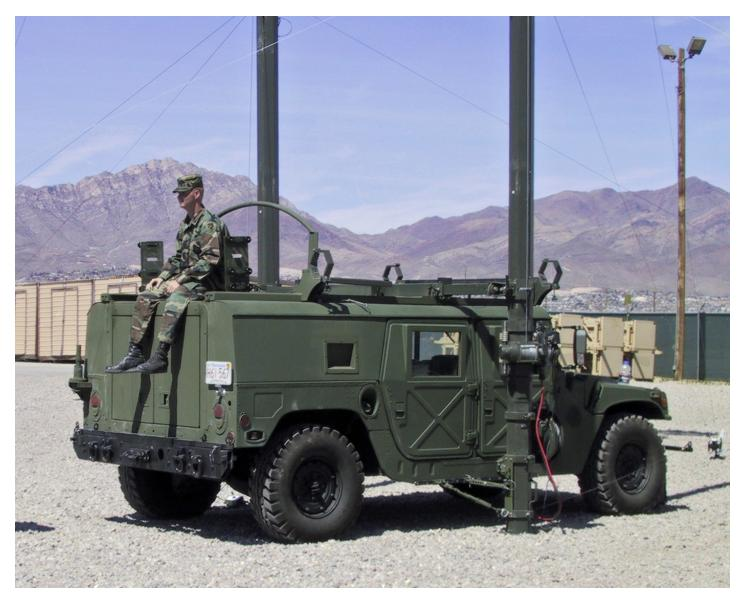
The MecPAM with its electric powered movement control with manual crank backup provides for the safe, speedy and precise deployment and recovery of 25 meter mast with heavy headloads up to 120 kg (264 lbs) by a crew of two.
