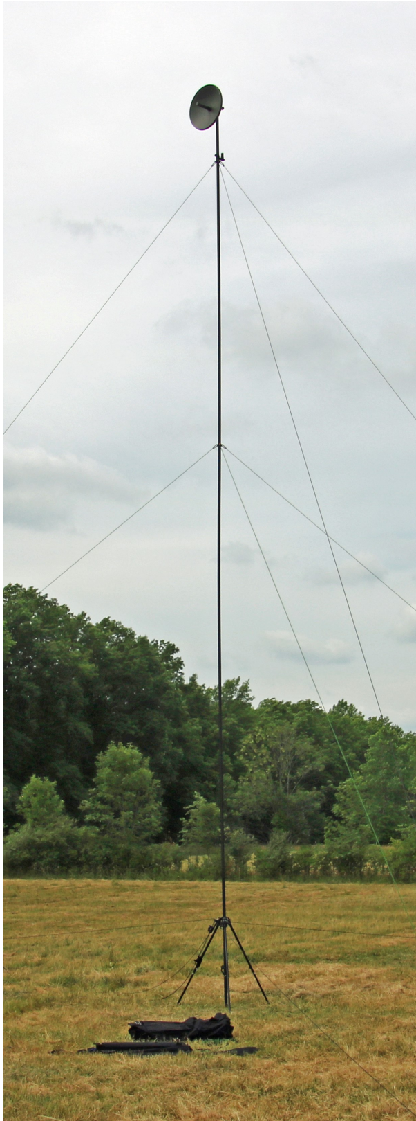
15 meter (50 ft) ULM-C 48/15-1.3 mast (shown supporting Comrod Band 4 dish antenna)
