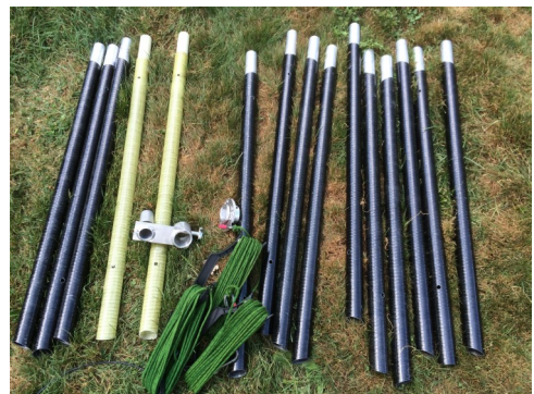
13 carbon fiber and 2 x glass fiber tube sections (2 x glass fiber sections will be painted black to match standard carbon sections)
