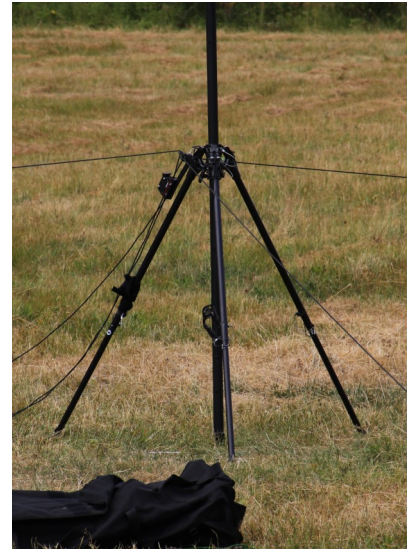
Tripod assembly with mast section hoist and lifting mechanism
