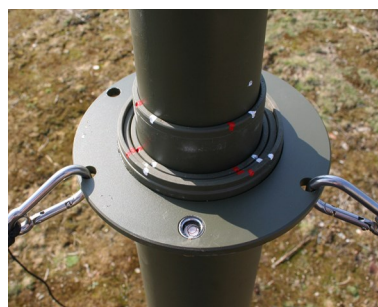
Bayonet tube locking system
