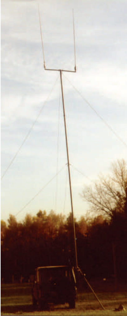
Sketch 1: 2 antennas on ULM-11/QESH mast
