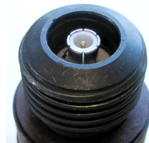
CEF connection on top of the base
