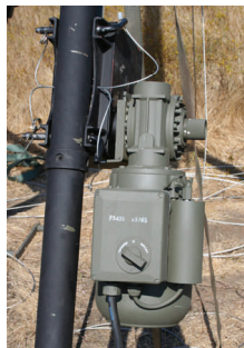
Electrical motor for lifting winch
