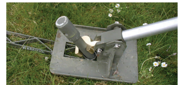
Stake remover for hard soils
