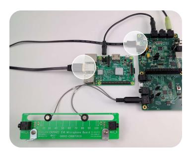
$\begin{array}{c|c} 4 & \text{Connect the audio path from micro USB (J1) to} \\ \text{USB port on RPi3} \end{array}$
