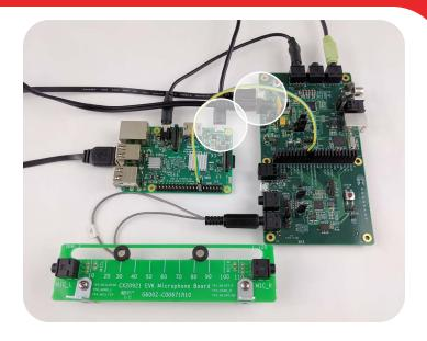
6 Connect the power supplies for both CX20921 evaluation board, (J10, +5V power supply included) and RPi3 (J1). Switch the power switch (SW3) to turn on the CX20921 evaluation board. LED D6 (5VLED) will turn on when there is power on the board.
