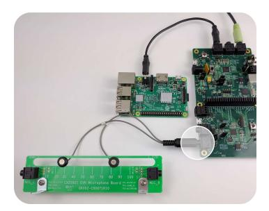
Connect the microphone module to the CX20921 evaluation board (J19)
