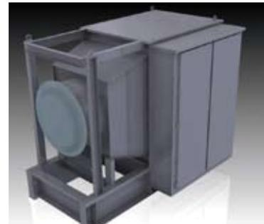
For brake resistors operating at more than 2kV, sheathed elements are unsuitable and we employ live elements. Normally, cooling is by simple natural convection, but if the heat losses after braking would impose unacceptable loads on the ship's air conditioning system we add an air-to-water heat exchanger to transfer the brake energy to the ship's chilled water system.
