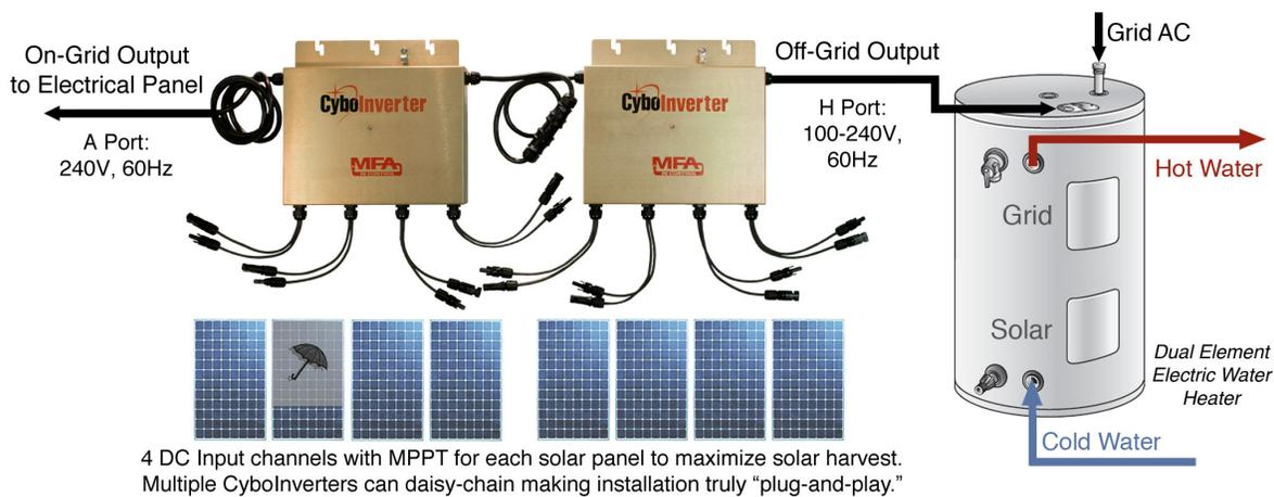
The following graphic shows a 4-channel 1.2KW On/Off-Grid CyboInverter that has an on-grid AC output port and an off-grid AC output port. Each inverter has four input channels that can connect to four 300W DC sources including solar panels, wind generators, or batteries and produce 1150W AC peak power. Each input channel has its own control and MPPT to eliminate solar partial shading problems and maximize power production. The product is patented, UL1741 certified,
