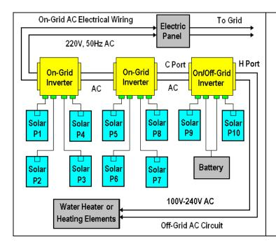
When the grid is on, the inverter works like a regular on-grid inverter that meets UL1741 and IEEE1547 standards including: over and under voltage shutdown; over and under frequency shutdown; and anti-islanding.
