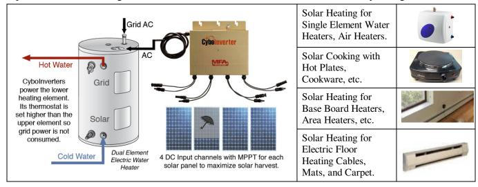
Product: 4 Channel 1.2KW Off-Grid CyboInverter for Electric Water Heaters Part No: CI-Mini-1200He Standalone Off-Grid Model, 100V-240V, 50/60Hz AC
