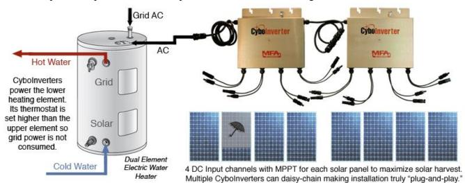
Product: Off-Grid CyboInverter H Model Twin Pack (Total 8 Input Channels)
