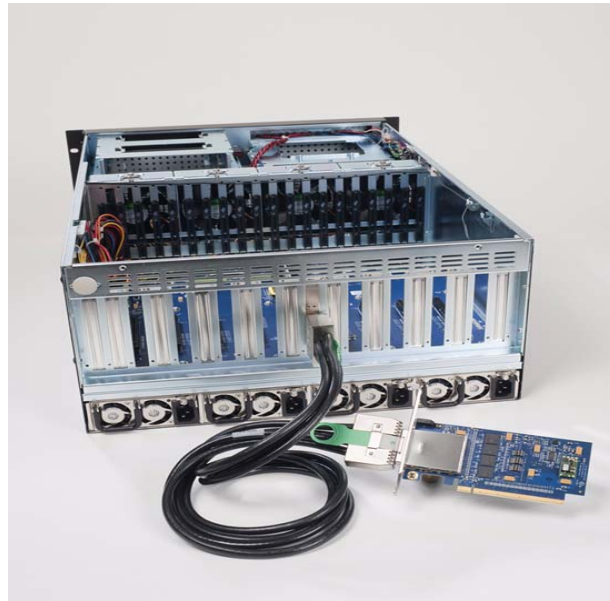
Figure 5-6. PCIe2-2709 5U Chassis
