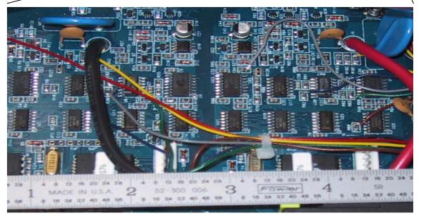
In the above design, a 736 array replaced 18 ICs and over 130 discrete components with a single 28L SOIC. Including design time, the entire cycle took 12 weeks with prototypes that worked first time. Board area: 8.3 sq. inches before, 0.225 sq. inches after.
