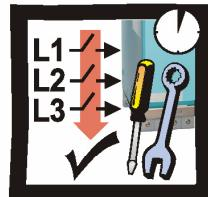
Before working on the unit, isolate the mains supply from terminals L1, L2 and L3 and wait 3 minutes.
