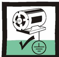
The drive motor must be connected to an appropriate safety earth.
