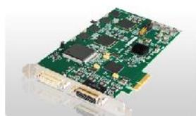
The XV-SD4+1s is the latest new video input module for the X-View DPX-E series of multi image display processors. XV-SD4+1s provides 4 SD video inputs which can be composite or Y/C format with support for PAL, SECAM and NTSC video, with full de-interlacing and real time 25/30 frames/sec display per input and 1 x DVI input that supports HD video to 1080P, VGA/RGB to 2048 x 1536 resolution.
