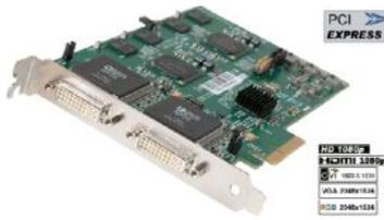
The XV-RGBE2s is the latest new video input module for the X-View DPX-E series of multi image display processors. XV-RGBE2s provides 2 DVI video inputs which can accept VGA/DVI/HDMI HD inputs for real time display across the video wall in a fully scaled and positioned window. *Note: HDMI HDCP & Audio is not supported.*
