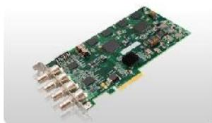
The XV-SDI2 is a dual channel PCIe HD-SDI video input module. The input module supports SD-SDI, HD-SDI and 3G-SDI (including 2K Digital Film Resolution modes).
