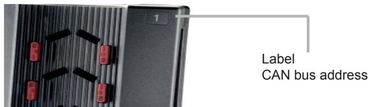
Figure 5: Labelling the CAN bus address on the module
