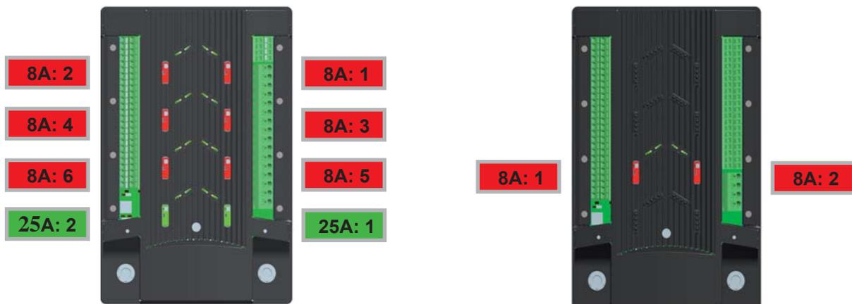
Figure 3: Circuit breaker identification on the modules
