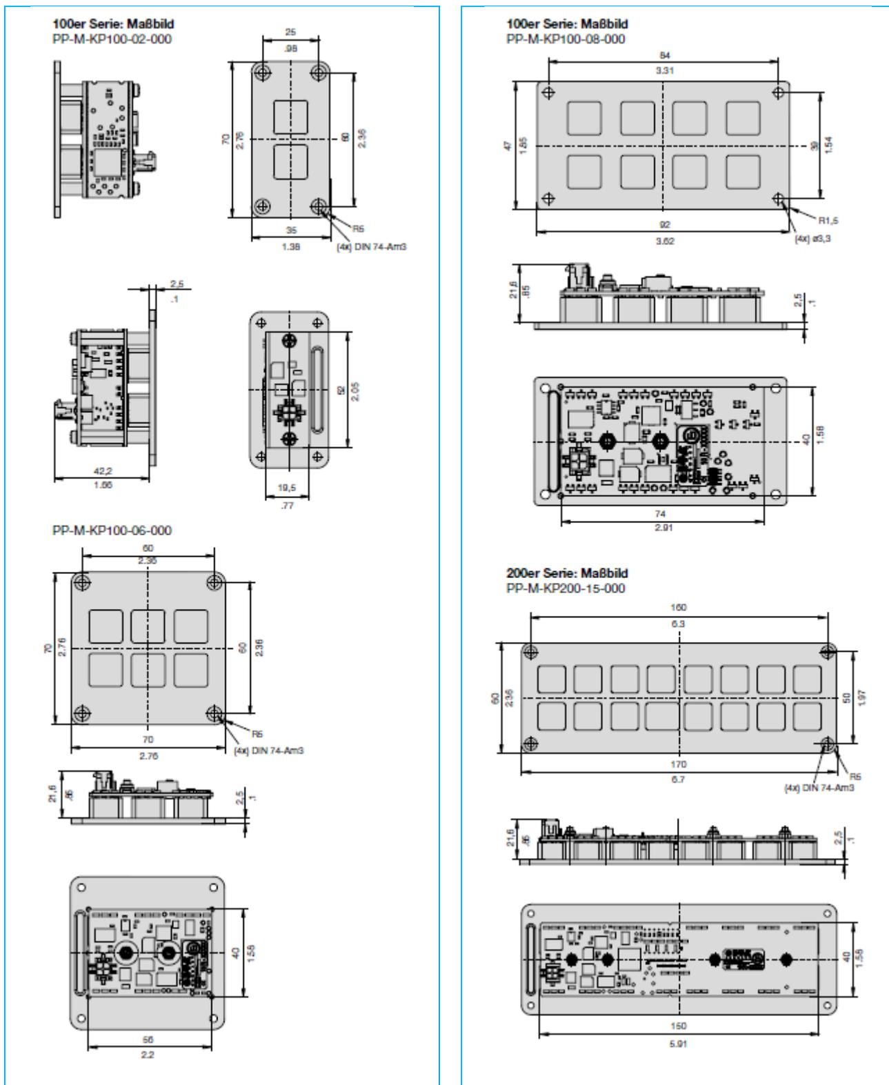
Fig. 7: Dimensions of the different PowerPlex® Keypads
