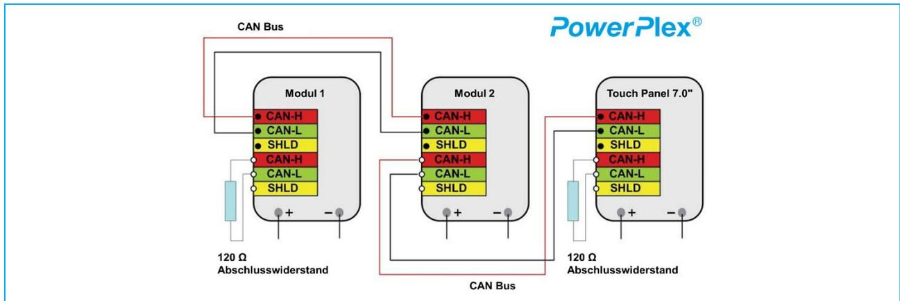
Fig. 9: Connection of the PowerPlex® components in the CAN bus system
