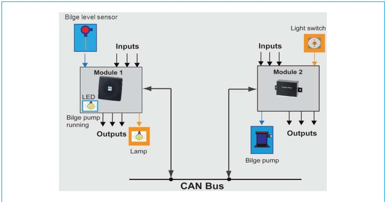
Fig. 3: Two PowerPlex® modules connected via CAN bus cable
