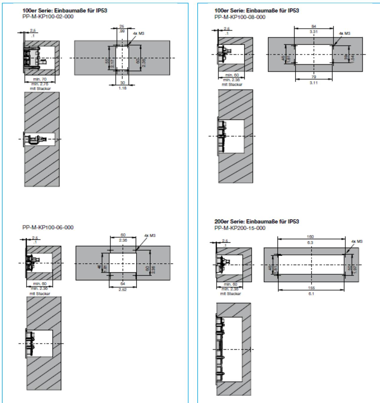
Fig. 6: Dimensions for the required mounting cut-out
