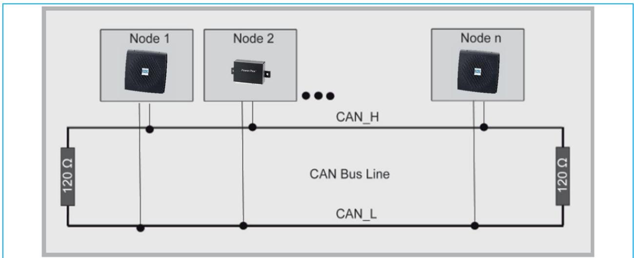
Fig. 4: Various PowerPlex® modules connected via serial CAN bus topology
