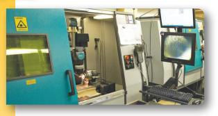
**Laser welding/cutting** - Eagle's computer controlled laser welding equipment (laser center shown above) enables us to produce extremely close-tolerance cutting, notching, etching and welding operations.
