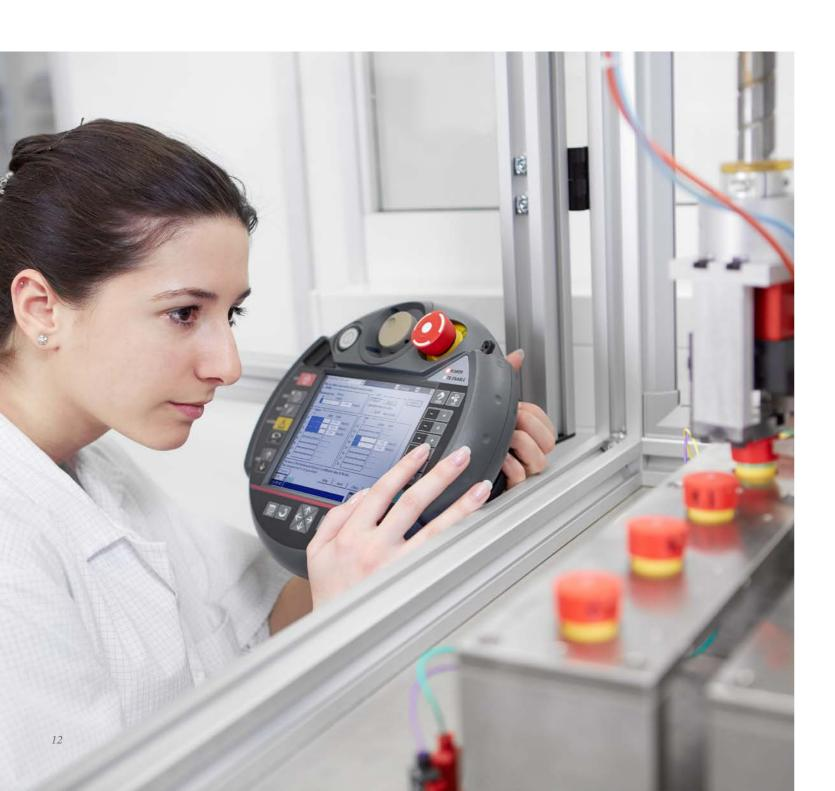
The demands placed on such handheld control devices can be greater than for built-in units. The environmental conditions in industrial settings require the utmost robustness and intuitive operation. HMI Components must not only withstand dirt and moisture, but also be intuitive to control.
