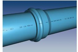
The Series 1900 is designed for restraining push-on PVC pipe bells. It has a split, serrated restraint ring on the spigot and a split serrated ring behind the bell.
