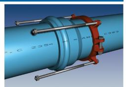
Remove the side bolts from the second serrated restraint ring. Use the Thrust Bolts to determine the proper location of the restraint ring on the spigot. Allow enough room on the thrust bolt to fully engage the nuts.
