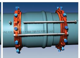
4. Position the restraint ring on the spigot or plain end such that the bolt holes are in alignment and the distance between the rings is suitable for the thrust bolt length. Allow enough room on the thrust bolt to fully engage the nut with several threads showing.
