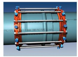
5. Install the thrust bolts in each available bolt hole for maximum distribution of operating forces. Place the nuts on the end of the thrust bolts. Allow enough room on the thrust bolts to fully engage the nut with several threads showing.
