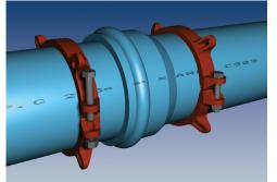
4. Install both halves of the restraint ring at the proper location, tapping each half into place. Make sure that the complete ID of the ring is touching the pipe before installing the side bolts. Tighten the side bolts evenly to 120 ft-lbs. (70 ft-lbs on 4" and 6")
