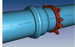
Install both halves of the serrated ring around the pipe behind the bell, tapping each half into place. Make sure that the complete ID of the ring is touching the pipe before installing the side bolts. Install the side bolts and tighten evenly to 120 ft-lbs. of torque. (70 ft-lbs on 4 inch and 6 inch)
