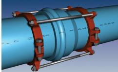
Place nuts on the thrust bolts and hand tighten until they are snug. Allow enough room on the thrust bolts to fully engage the nuts. Do not tighten these bolts enough to force the spigot further into the bell of the joint.
