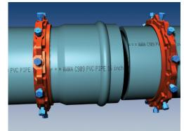
The Series 2916 is designed for restraining AWWA C909 PVC Pipe with push-on bells. It has one restraint ring behind the bell and on the plain end.
