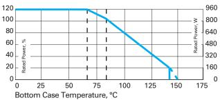
Derating (thermal resist.) UXP 800: 9.09 W/°K (0.11°K/W) Power rating: 800 W at 85°C bottom case temp.\* Please ask for detailed mounting procedure!
