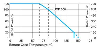
Derating (thermal resist.) UXP 600: 8.33 W/°K (0.12°K/W) Power rating: 600 W at 85°C bottom case temp.\* Please ask for detailed mounting procedure!
